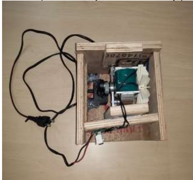
Fig:-1 220 V micro AC single phase Compact Portable Compressor
